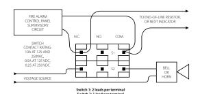
NOTE: The above diagram shows a connection between the common terminal (yellow - S1 and yellow-with-orange stripe - S2) and the normally closed terminal (blue - S1 and blue-with-orange stripe - S2). In this example, the indicator light and alarm will stay on until the valve is fully open. When the valve is fully open, the indicator light and alarm will go out. Cap off any unused wires (e.g. brown with orange stripe).
