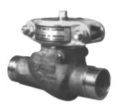
Available with Type 316 stainless body and trim in the 2" (50 mm) size, Swinger check valves are supplied with bonnet cap drilled and tapped with ½" (12.7 mm) NPT pipe plug for chemical injection or other auxiliary connections.
