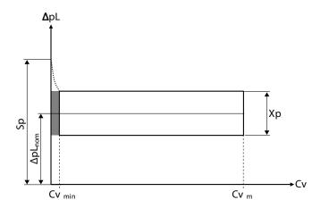
Sp = Sealing pressure, the increase of  $\Delta pL$  in psi when a  $\Delta p$  controller controls  $\Delta pL$  from  $Cv_{min}$  down to zero flow.
