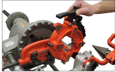
5. Lower the threading head onto the pivot adapter assembly, checking for proper alignment.
