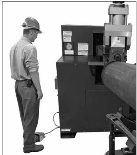
12. To start the grooving operation, depress and hold down the safety foot switch. This will advance the upper roll into contact with the pipe. The lower roll will start rotating, and the groove will begin to form.
