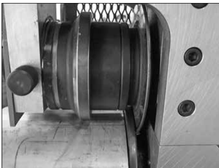
10. Insert a length of pipe that is the correct size, material, and thickness onto the lower roll. Ensure that the pipe end contacts the lower-roll backstop flange completely. Remove hands from the pipe.
