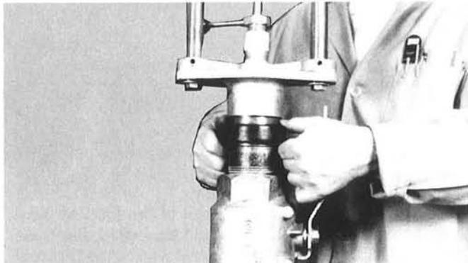
6. Slide the HP-70 Gasket into position centered between the grooves on the base unit and grooved pipe as shown. No portion of the gasket should extend into the groove on either the grooved pipe or the base unit.
