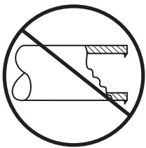
Unacceptable pipe end with burrs
